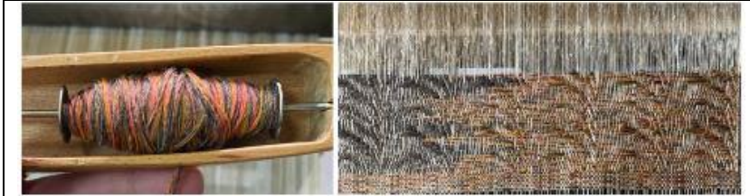
Figure 4. The effect of weft yarn prepared with yarns of different colors on weaving
