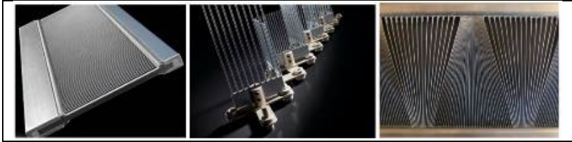
Figure 6. Normal and special design reeds (Blureed; Rios)
